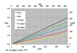
For microglass absolute-rated media, the  $\Delta P$  will be approximately 10% lower than polypropylene media. For 40" filter elements, expect the pressure drop to be 20-30%, higher, on average, than depicted in the flow chart above.
